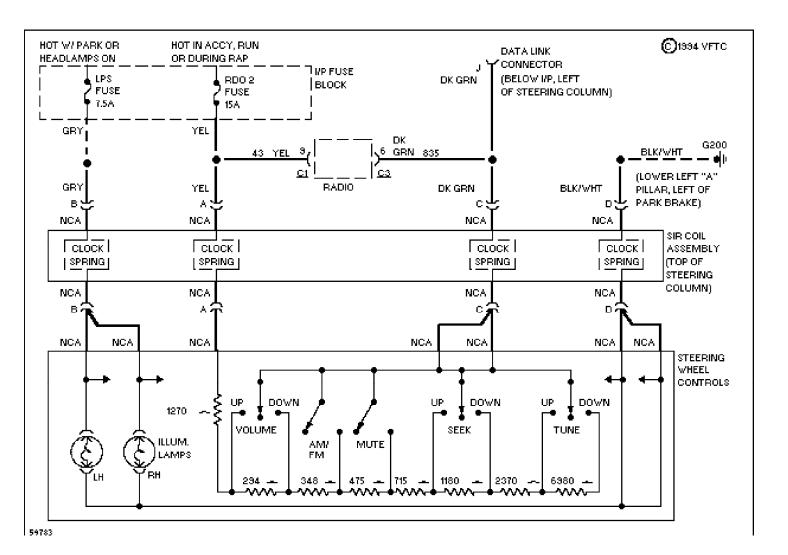
SYSTEM WIRING DIAGRAMS 3.8L (VIN L), Data Link Connector Circuit (p. 4) 1994 Pontiac Trans Sport
