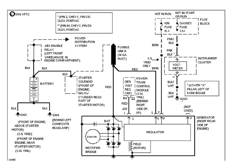
SYSTEM WIRING DIAGRAMS 3.8L (VIN L), Starting Circuit (p. 41)
