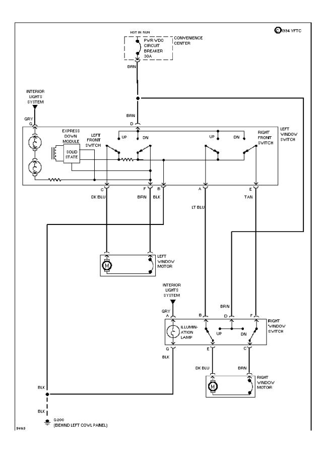
SYSTEM WIRING DIAGRAMS
