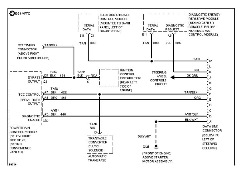
SYSTEM WIRING DIAGRAMS Steering Wheel Controls Circuit (p. 3) 1994 Pontiac Trans Sport
