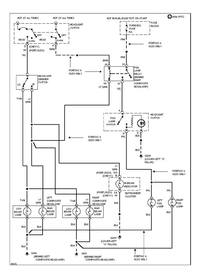
SYSTEM WIRING DIAGRAMS Headlamps Circuit, W/ DRL (p. 21)
