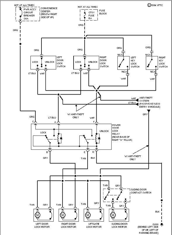
SYSTEM WIRING DIAGRAMS Door Lock Circuit, Automatic Door Locks (p. 32) 1994 Pontiac Trans Sport
